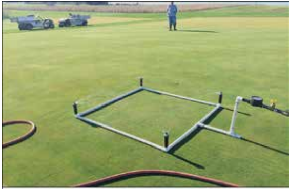
Irrigation simulator used to precisely apply post-application irrigation after fungicide application.
