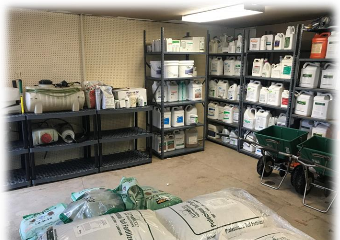
Figure 9-1. Chemical storage with pesticides and fertilizer stored separately on metal shelving at Bogey Hills Country Club (St. Charles, MO).
