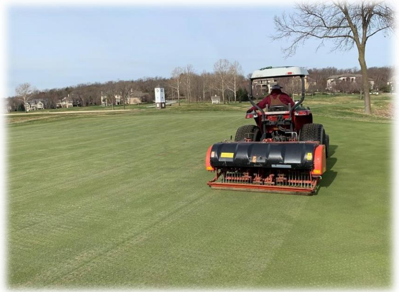
Figure 7-1. Using a deep tine aerator on the green surface at The National Golf Club of Kansas City
